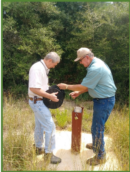
Greg Sengelmann and Jim Benedict, GCUWCD setting transducer at monitoring well
