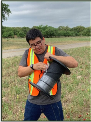
Omar changing out transducer at Monitoring Well MW-CZ-7
