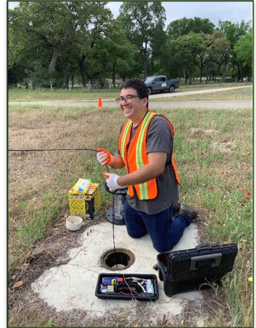
Omar changing out transducer at Monitoring Well MW-CZ-7
