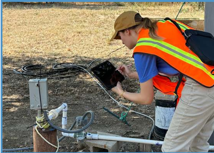
Pictured above: Caroline using iPad to record September water level data into mobile survey app
