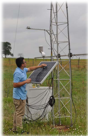
Pictured here: Omar cleaning solar panels at weather station
